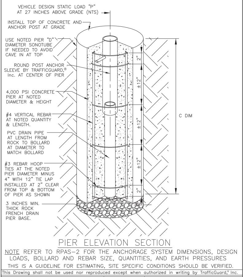
THIRD ANGLE PROJECTION ROUND POST BOLLARD RPAS TrafficGuard,® Inc. Toll ANCHORAGE SYSTEM ASSEMBLY Do not scale from drawing Free P.O. Box 201, Geneva, IL. 60134 Bus: 1.877.727.7347 Fax: 1.800.814.7194 Action wkz Dwg. Scale: nts Assembly Shipping Weight Drawing Number: Design wkz|Copywrite: 2010| Varies per Model|RPAS-1 1 \_ Checked wkz Dwg. Size: Letter Drawing Date: 12.10.10 Sheet: 1 of 2 Date Description
